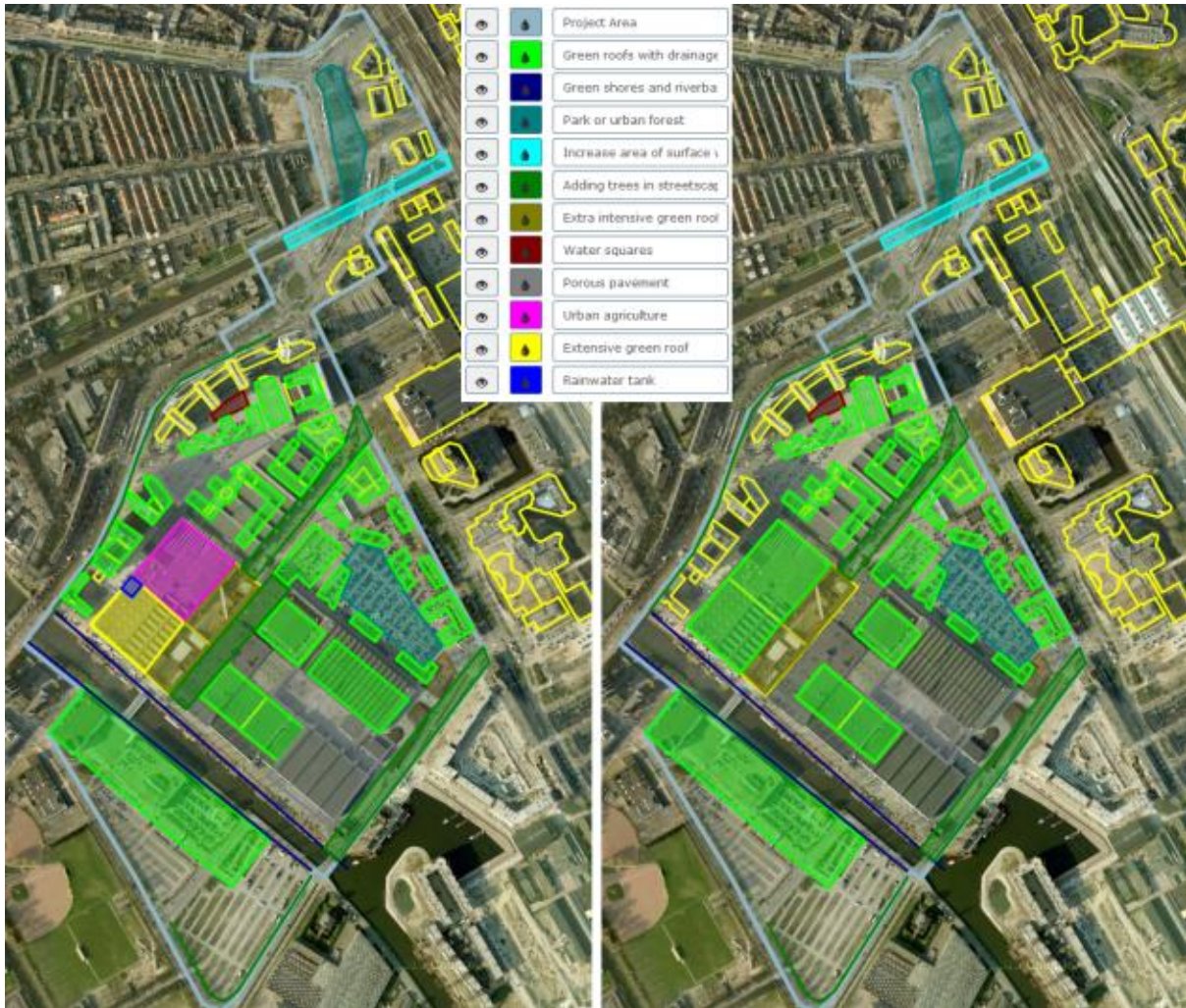
Figure 4 Example of AST application: Two of the alternative conceptual adaptation plans for the Utrecht City Centre - West, each with its own set of adaptation measures and, consequently, a different contribution to adaptation targets and co-benefits. The Green alternative (right) proved less effective than the Plus alternative (left)[Van de Ven et al. 2016]
