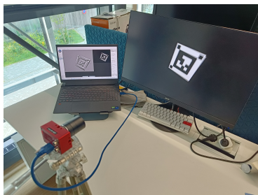
Figure 3.8: Filming MKV with an event camera, event frame output can be seen on the left screen.
