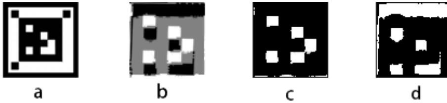
Figure 3.15: A: marker M_c , B: the marker candidate extracted from M_c . C: M_c 's on-event candidate. D: M_c 's off-event candidate, the large white area on the top of this image is the white frame of our marker.
