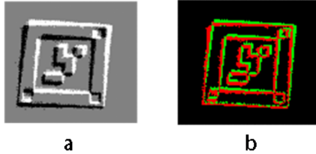
Figure 5.1: A: the event frame of a marker moving towards the top left, B: events are divided into two groups according to their timestamps, where red pixels are old events and green pixels are new events. The moving direction can be seen from B.
