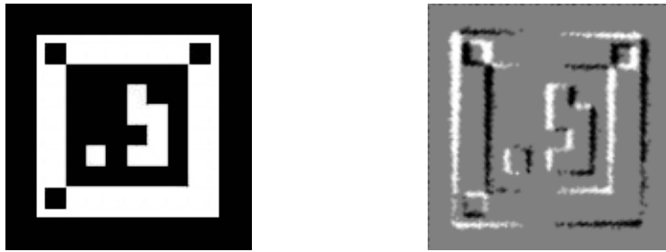
Figure 3.2: Optimized fiducial with its direction indicator (black blocks on the white frame), and an output view of an event camera.
