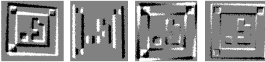
Figure 3.5: An output with continuous contours(first), discontinuity caused by unidirectional shift, rotation, and slow movement (second, third and fourth). The edges of the markers are not connected anymore.
