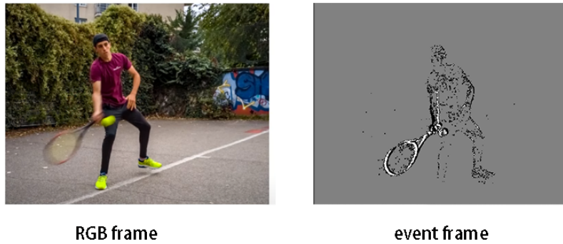
Figure 2.3: Comparison between the RGB frame of a frame camera and the event frame of an event camera. In the event frame, white and black pixels represent the on and off of events. Gray pixels indicate that no event has been triggered or the overlap area of on and off events. It can be clearly seen that the outline of the high-speed swinging racket is blurry in the RGB frame but clear in the event frame. [36]
