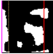
Figure 4.14: An incorrect first refinement result. The purple solid line is the correct calculated position of the left edge of the white frame, the red line is the incorrect calculated position of the right edge of the frame, and the yellow dotted line is the manually added expected right edge position.
