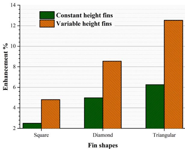
Fig. 16. Solidification enhancement percentage for different fin shapes.
