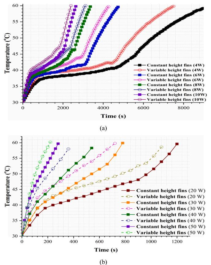
Fig. 5. Heat sink base temperature against time intervals for various heat inputs.
