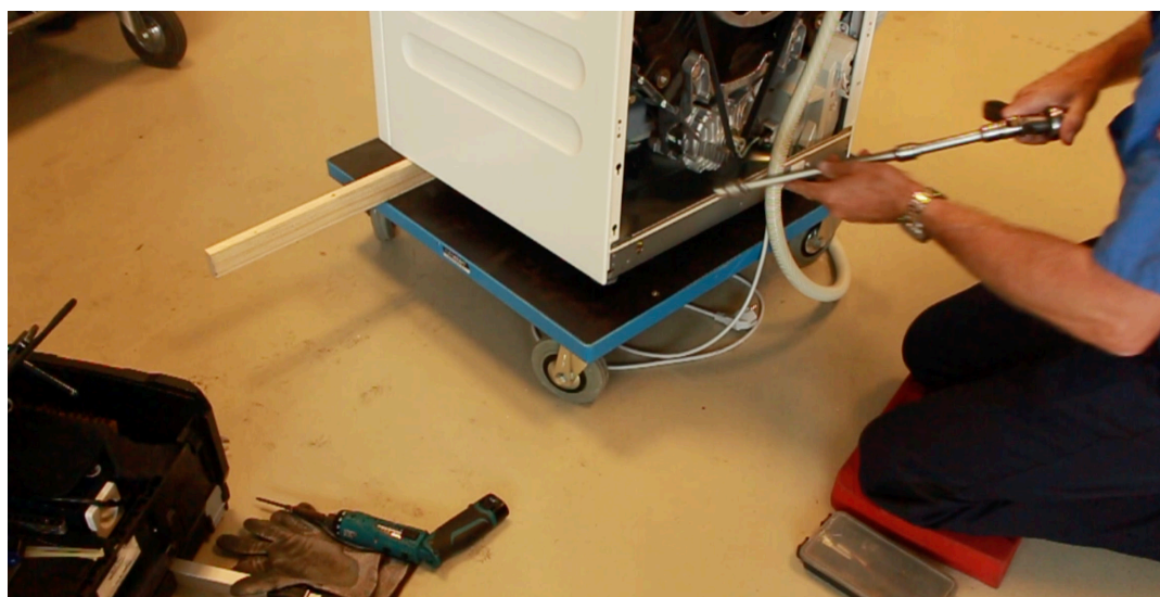
Image 16. Tool extension needed to reach the component.
