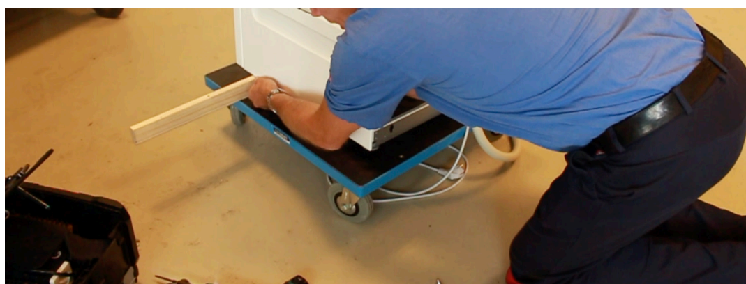
Image 17. Lack of visibility and extension of both arms needed to reach and release the component.
