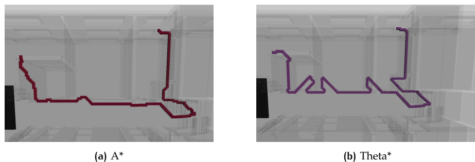
Figure 6.2: Path zigzagging in Theta*. The zigzagging near doors is very extreme with Theta*.
