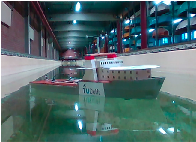
Figure 3. 'Grey Seabax' model scale offshore vessel.
