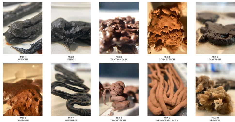
Fig. 2 Material Experimentations in a hot and cold extrusion process (Pictures by authors)
