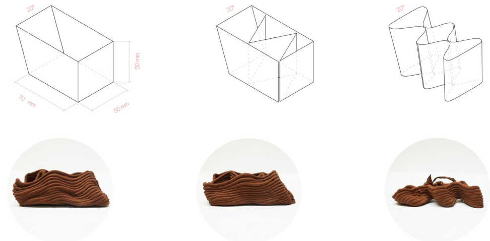
Fig. 13 Overhand testing (pictures & diagrams by authors)
