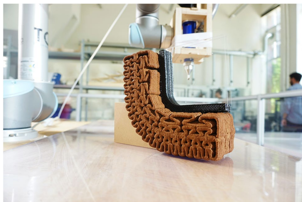
Fig. 14 Window frame final prototype (picture by authors)
