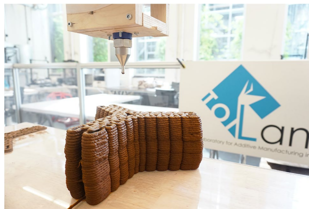
Fig. 15 Structural Node Final Prototype (picture by authors)
