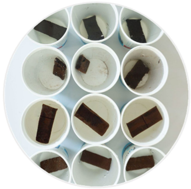
Fig. 5 Water absorption & retaining test (picture by authors)
