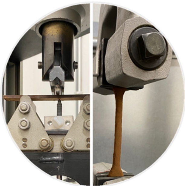
Fig. 4 Tensile & 3 point bending test (picture by authors)
