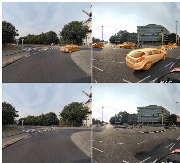
Figure 1: Example of moving object segmentation (top) and the results after inpainting (bottom). The regions that are highlighted in orange are removed and inpainted.
