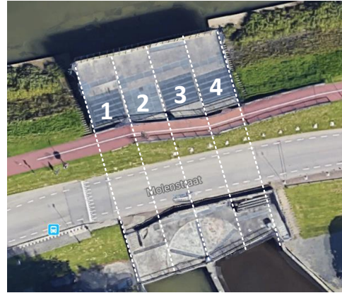
Figure 1: Top view of the Elshoutsluice including marking of the culverts. River is at top side of figure (source: Google maps).
