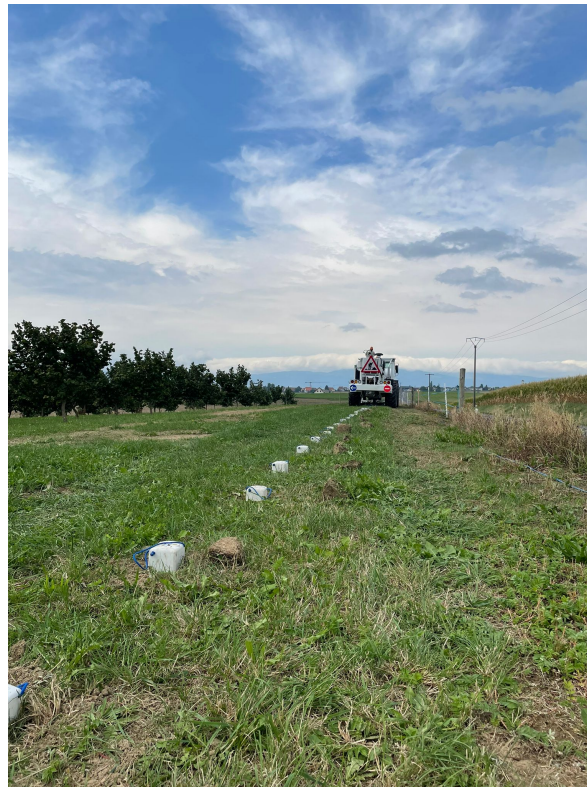
Figure 2-2: Acquisition for my internship project at Geo2x. 3D wireless geophones were placed along a line. The source was the vibrator truck, called "MiniVib", which swepted the input signal on the field from an offset position by changing frequencies and drive levels from 5% to 80% and downwards,too.
