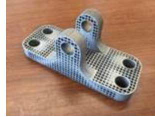
(b) Variable-density periodic lattice infill [20]
