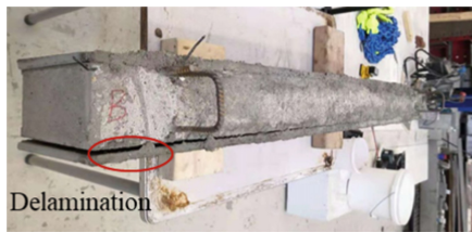
Fig. 6. Interface delamination for cast in-situ strengthened beam.
