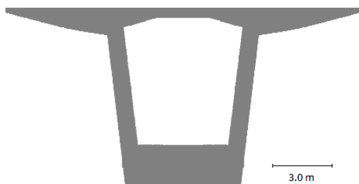
Figure 4.1: Cross section of the Hollandsch Diep bridge
