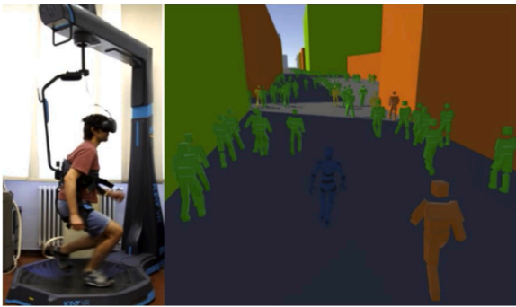
Fig. 9. Simulation of an evacuation procedure using virtual reality. The color of each agent indicates her health conditions.
