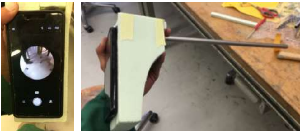
Fig. 2 Foam holder for laparoscope and smartphone, to capture the view from the laparoscope.
