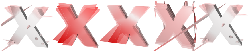
Figure 5.10: Compressed vibration modes produced by using ADMM for \mu = 10, 20, 30, 50, 75 . See Figure 5.1 for the output of our method.
