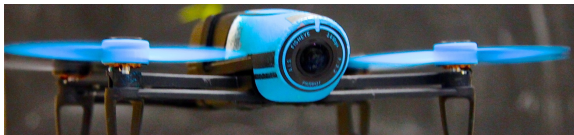
Figure 5.6: A Parrot Bebop 1 is used as the flying platform. The original autopilot is fully replaced by an open-source autopilot called Paparazzi UAV.
