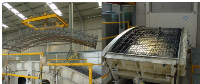
Figure 4.16: RC reinforcement cage [34]
