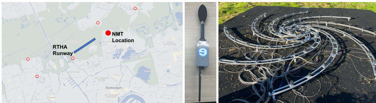
Figure 2: (left to right) RTHA with NMTs where the red dot represents the location of the chosen NMT, and the blue line represents the runway; Portable munisense microphone; 2D array with 64 microphones.
