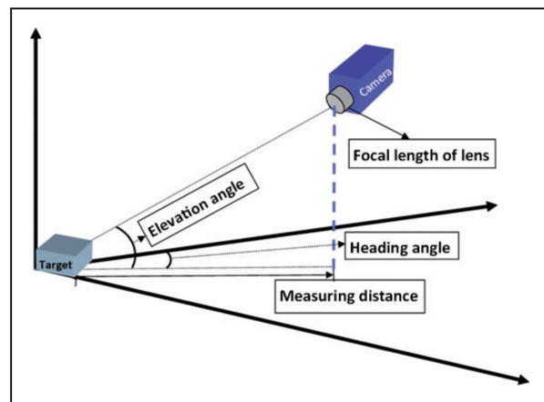
Figure 4. Illustration of the operational parameters.
