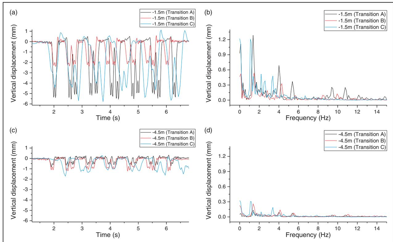
**Figure 13.** Rail vertical displacement of Transition B at  $-1.5$  and  $-4.5$  m compared with Transition A.
