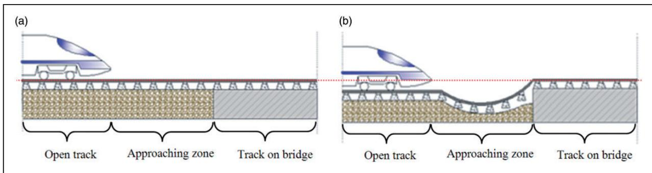
**Figure 2.** Schematic diagram of the differential settlement in the transition zone: (a) immediately after construction or maintenance (no settlement) and (b) after a few months of operation.
