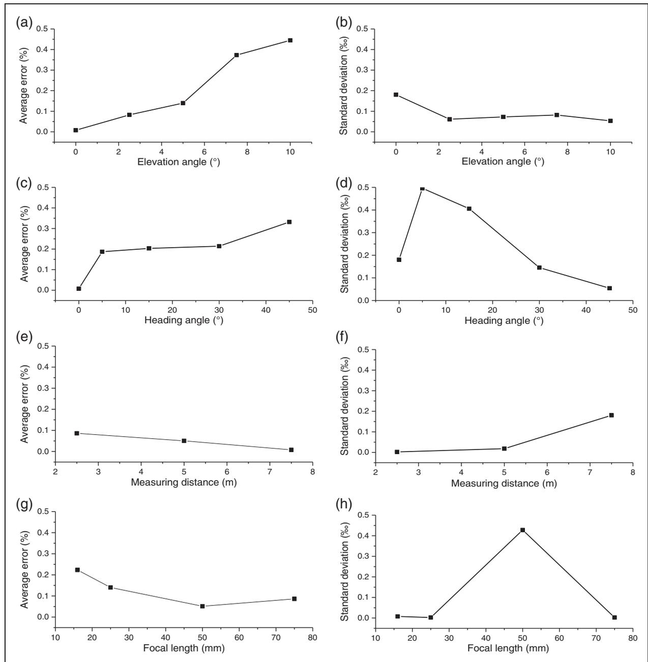
**Figure 5.** Effect of the elevation angle: average error (a) and standard deviation (b), effect of the heading angle: average error (c) and standard deviation (d), effect of measuring distances: average error (e) and standard deviation (f) and the effect of focal length: average error (g) and standard deviation (h).
