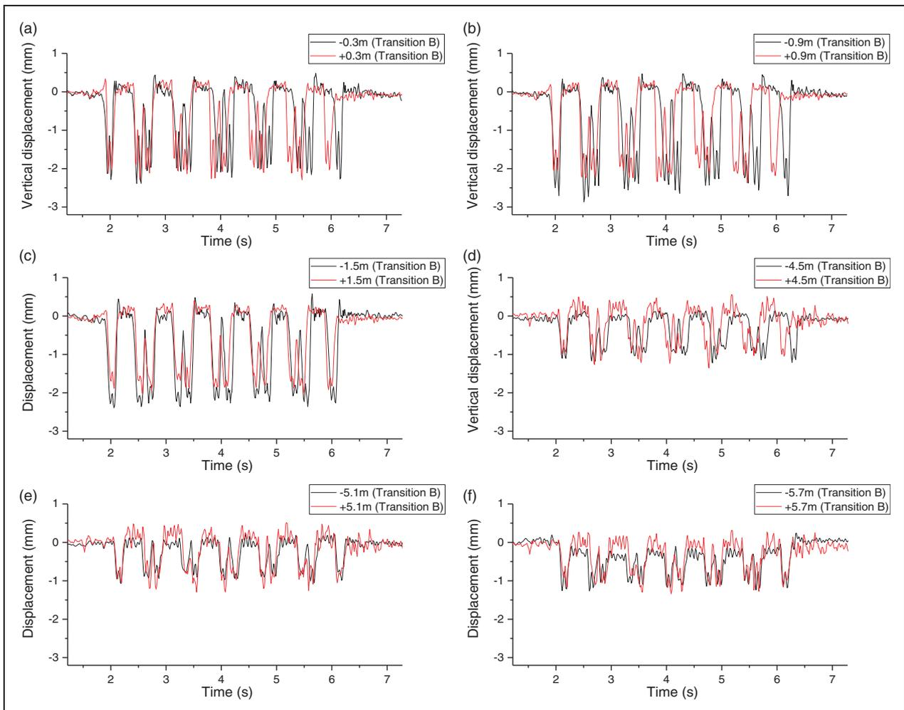
Figure 11. Rail vertical displacements in the embankment–bridge and the bridge–embankment transitions of Transition B.
