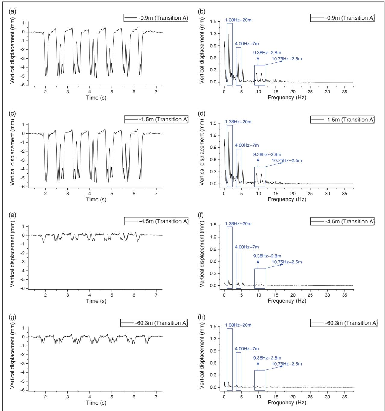
**Figure 9.** Rail vertical displacements at four locations of Transition A in the time domain (a), (c), (e) and (g) and in the frequency domain (b), (d), (f) and (h).
