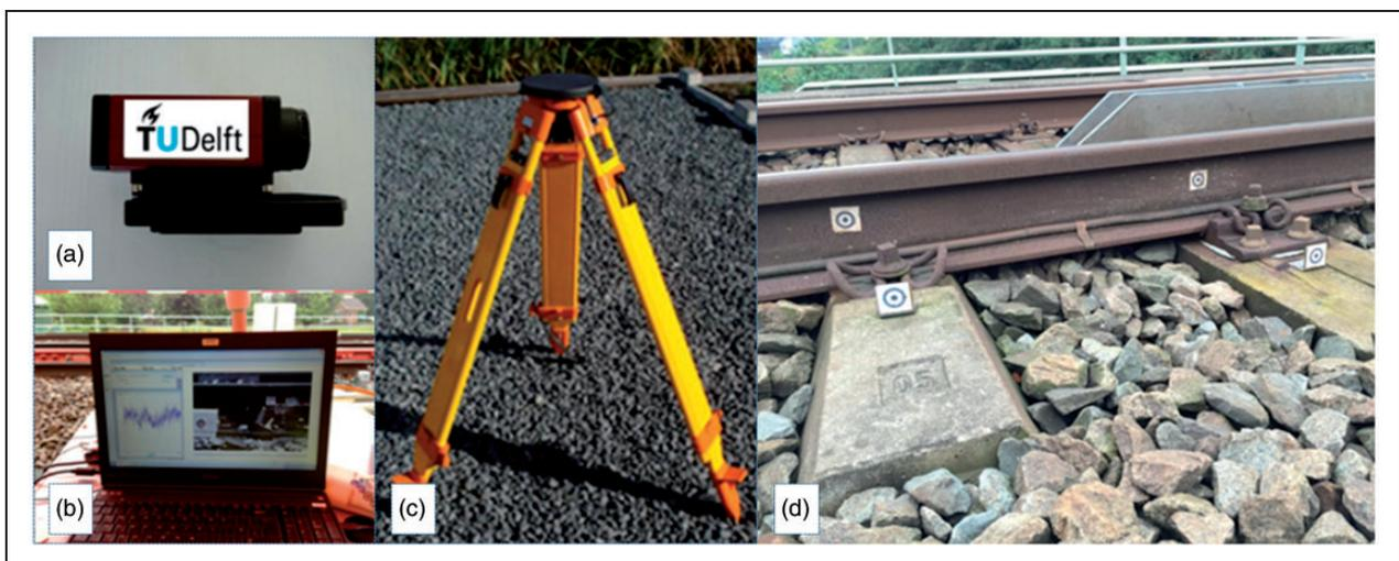
Figure 3. Components of the DIC-based device: (a) a high-speed camera, (b) the processing system, (c) a tripod and (d) targets.
