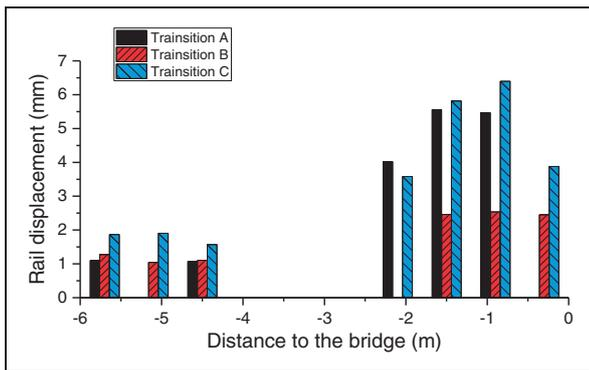
**Figure 14.** Comparison of vertical rail displacements in the approaching zone of two transitions.
