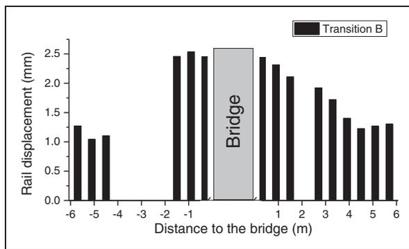
**Figure 12.** Statistics of the vertical rail displacements at all measured points of Transition B.
