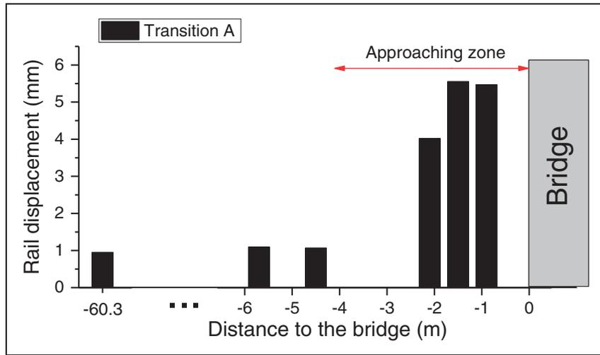
Figure 10. Statistics of the vertical rail displacements at all measured points of Transition A.
