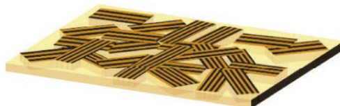
Figure 2.18: Tow-based discontinuous composite representation [47].
