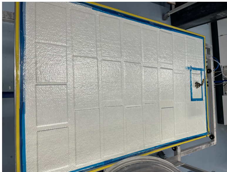
Figure 4.15: Laminate manufacturing's prepared vacuum bag.
