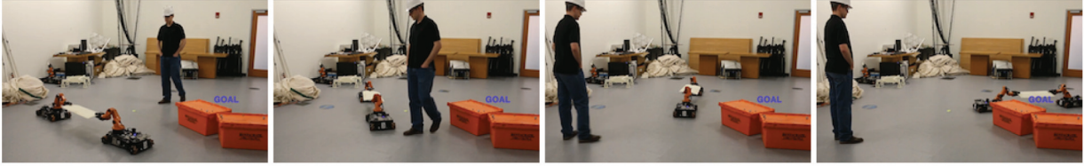
Fig. 12. Four consecutive snapshots of an avoidance maneuver where two mobile manipulators collaboratively carry a rigid object and navigate it to the goal while adjusting their formation to avoid collisions with the orange boxes and the human. Robots and human are tracked by overhead cameras. This maneuver is performed in 1 minute.
