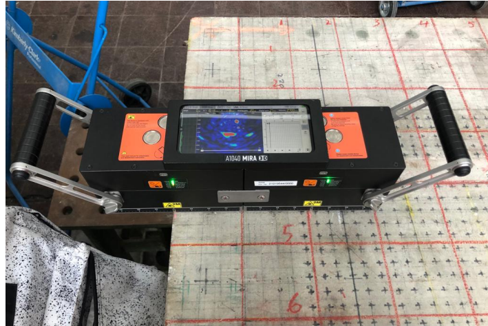
Figure 3-4: Photo of the device position for noise trace testing
