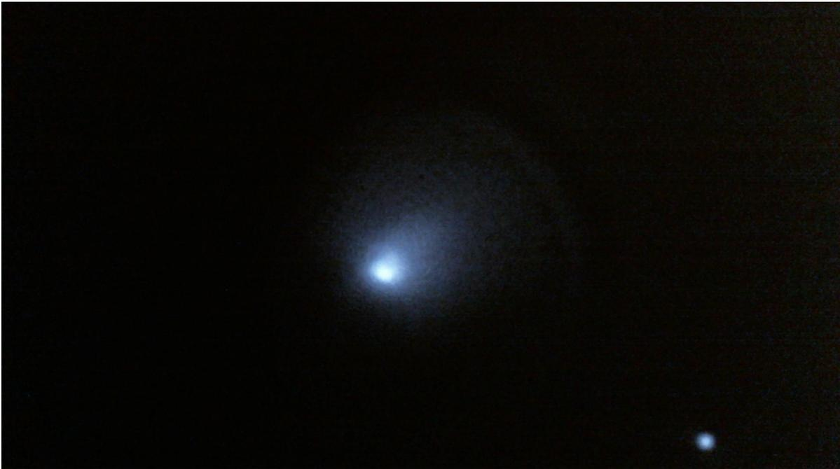
**Figure 5.53:** Image captured by the acquisition sensor during a link acquisition test, with the main incoming beam in the centre and a ghost beam in the bottom right of the picture.
