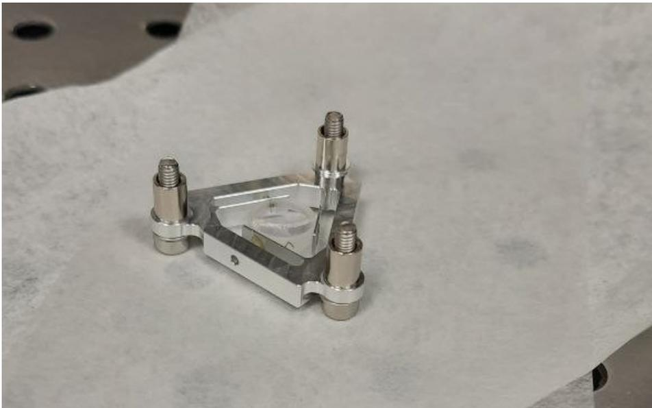
**Figure 4.6:** Lens focusing the incoming beam on the detector with spacers for fine alignment.
