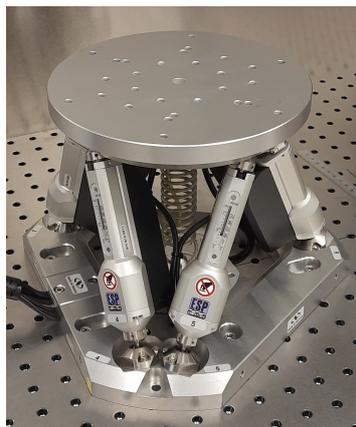
**Figure 5.52:** Hexapod used in the OFMT setup.
