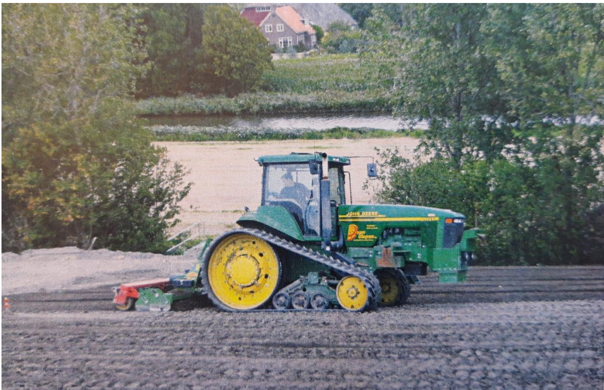
Figure 37: Loosening of the soil using a tractor with spades.
