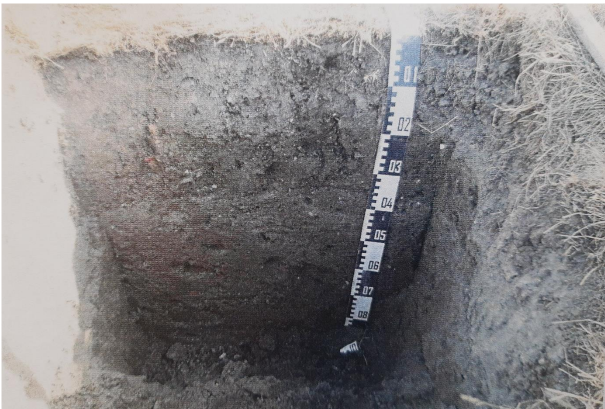
Figure 48: Excavation August 2013: Soil profile (Melchior+Wittpohl, 2014a). Clear signs of soil aggregation, especially in the top 40 cm.
