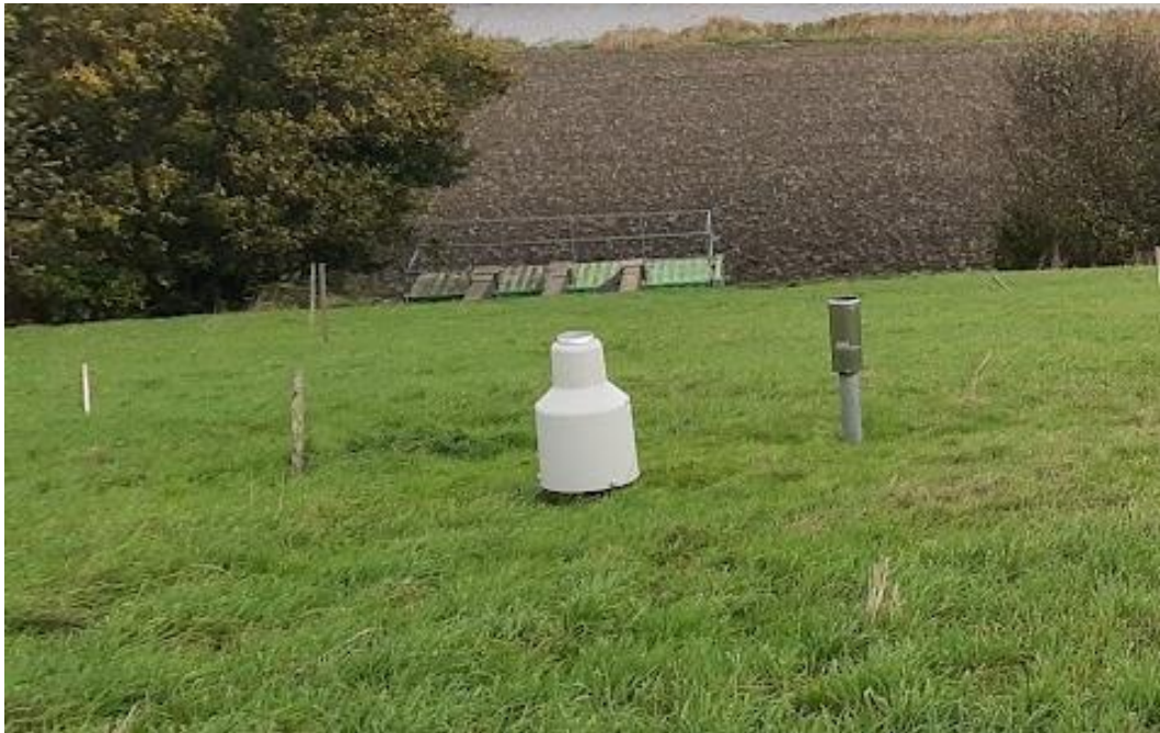
Figure 40: Three rain gauges at the test field as seen from the top of the field. In front the white Pluvio-2 rain gauge, to its left at the wooded stick the manual rain gauge at ground level and to its right the manual rain gauge at 1 meter height.
