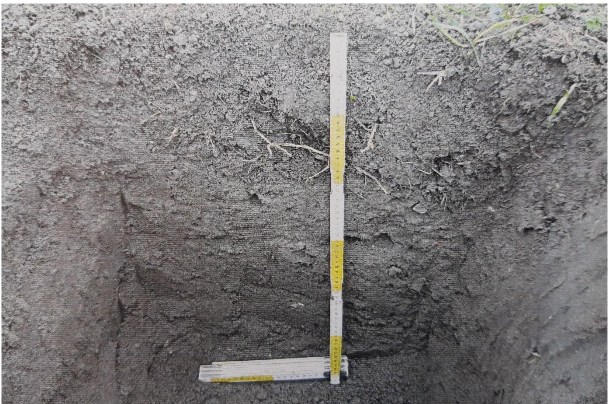
Figure 50: Excavation September 2013: Soil profile. Rooting of newly growing grass is strongest to 20 cm depth (Melchior+Wittpohl, 2014a)
