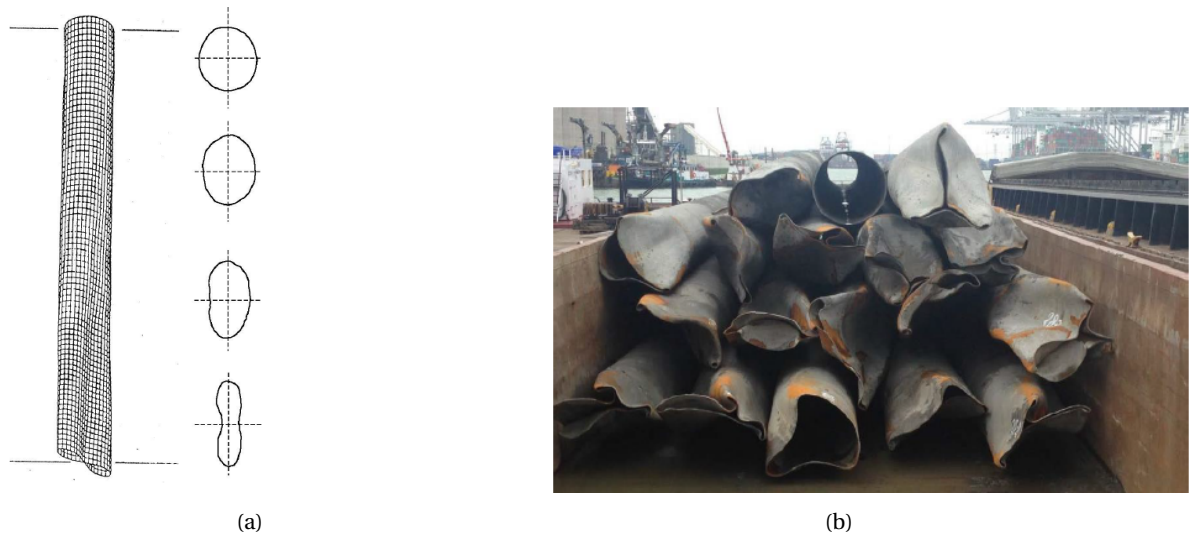
Figure 1.3: (a) Goodwyn A primary pile collapse details (Erbrich et al., 2011). (b) Removal of a quay wall in Rotterdam (cited by Cathie associates, 2017). Piles driven into dense Pleistocene sand with a D/t of 75.
