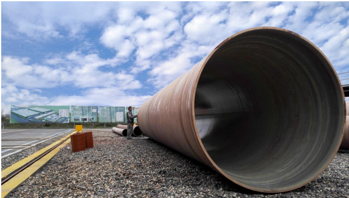
Figure 5. These long-life drainage pipes can replace steel. Credit: ERCBWC.
