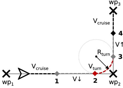
FIGURE 3. Turning manoeuvre as simulated within BlueSky.
