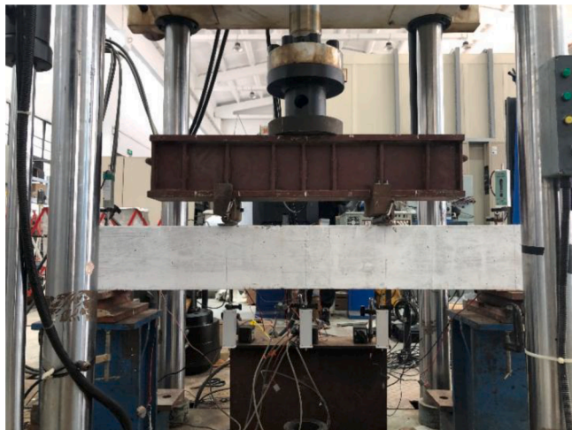
Fig. 5. Monotonic four-point loading of CFRP-strengthened RC beams.
