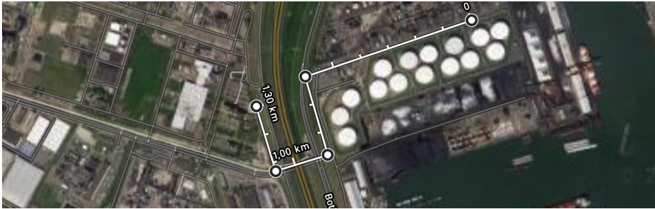
Figure A.12: Length estimation of the first part of the Steam Pipe, connecting Air Liquide and Huntsman (Google Maps).
