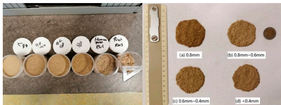
Figure 1. Appearance of reed fiber (0.8 mm, 0.6 mm to 0.8 mm, 0.4 mm to 0.6 mm, and less than 0.4 mm).
