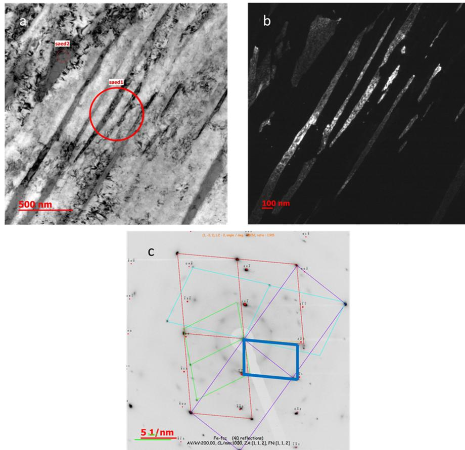
**Figure 4.** (a) Bright-field TEM observation of the quenching and partitioned (Q & P) steel. The red circles show the aperture positions from where the selected area diffraction (SED) patterns were obtained to identify the BCC and the FCC phases. (b) Dark-field image based on the FCC diffraction spots, showing the interlath retained austenite (white). (c) Diffraction spots in which the peaks corresponding to FCC are indicated by the blue lines.
