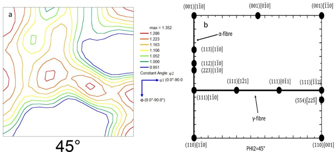
**Figure 5.** (a) Orientation distribution function (ODF) of the material of which the  $\phi_2 = 45^\circ$  section is presented; (b) a schematic representation of the  $\Phi_2 = 45^\circ$  section of the Euler space showing the main BCC texture components.
