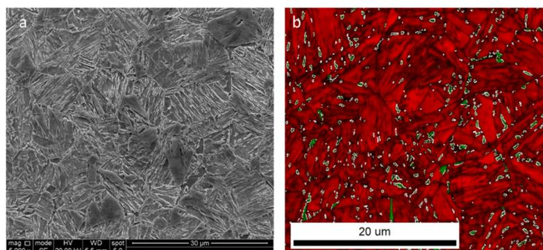
**Figure 3.** (a) Secondary electron SEM image and (b) combined image quality (IQ) and phase EBSD maps showing the BCC phase (martensite) in red and FCC phase (austenite) in green. Grain boundaries that fulfil K-S orientation relationship are in white.
