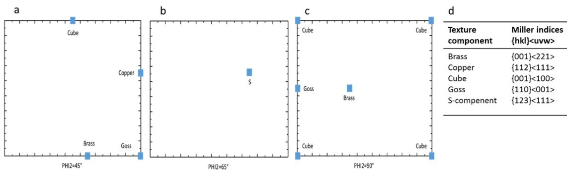
**Figure 7.** A key for the main texture components in FCC metals. (a)  $\Phi_2 = 45^\circ$ ; (b)  $\Phi_2 = 65^\circ$ ; (c)  $\Phi_2 = 90^\circ$  and (d) a table with the Miller indices of the main texture components.
