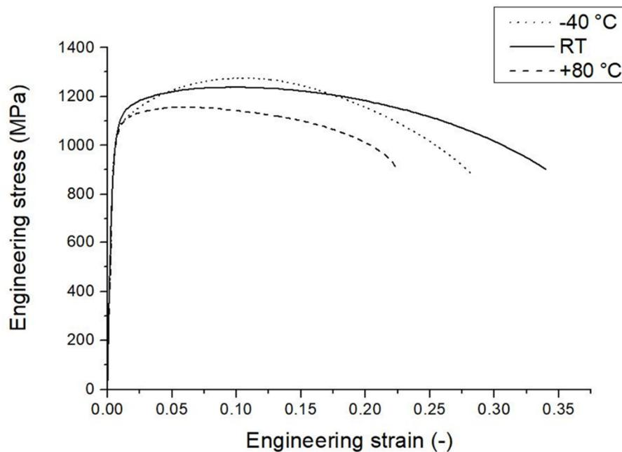
**Figure 10.** Static engineering stress-strain tensile curves obtained at  $-40\text{ }^{\circ}\text{C}$ , RT and  $80\text{ }^{\circ}\text{C}$ . The tests were carried out with the gauge section parallel to the rolling direction.
