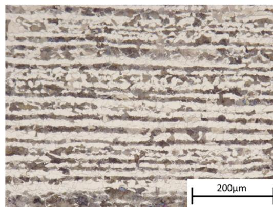
**Figure 2.** Light optical microscopy image of the steel after hot rolling.
