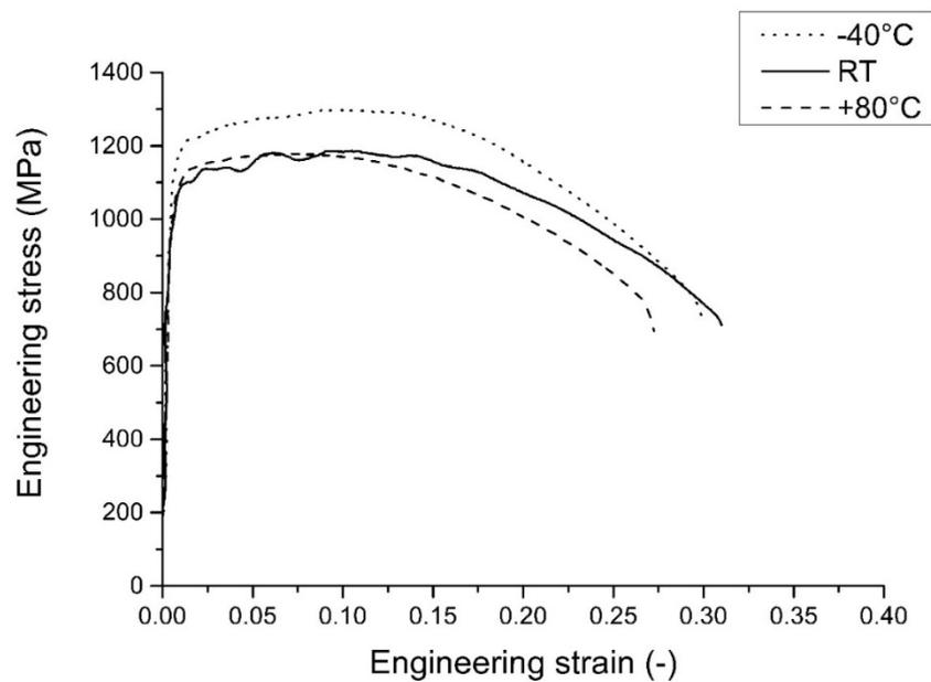
**Figure 12.** Engineering stress-strain curves of the material tested under dynamic conditions at  $-40\text{ }^{\circ}\text{C}$ ,  $20\text{ }^{\circ}\text{C}$  and  $80\text{ }^{\circ}\text{C}$ . The tests were carried out with the gauge section parallel to the rolling direction.
