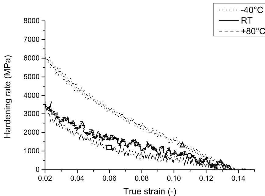
**Figure 11.** Hardening behaviour for tests performed at  $-40\text{ }^{\circ}\text{C}$ , RT and  $80\text{ }^{\circ}\text{C}$ . The end of uniform straining is indicated by a triangle, circle and square for, respectively, the experiments carried out at  $-40\text{ }^{\circ}\text{C}$ , RT and  $80\text{ }^{\circ}\text{C}$ .
