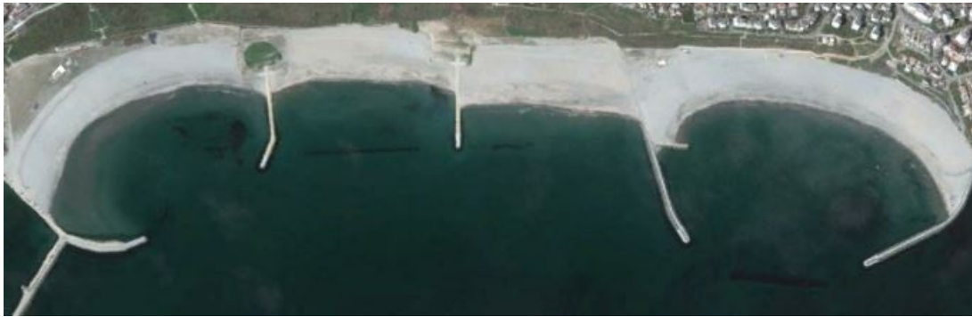
Figure 5.3: Overview of the layouts of Tomis Centre and Tomis South beaches (North is right) (Google Earth Pro V7.1.8.3036, 2016a)
