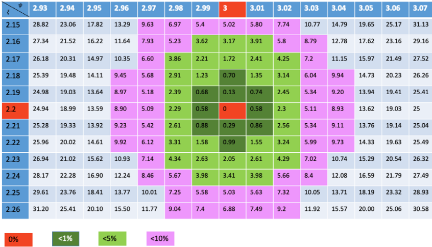
Figure 4.19: Relative error on the degree of polarization (%) as a function of the uncertainty on the apex angles \xi and \psi .
