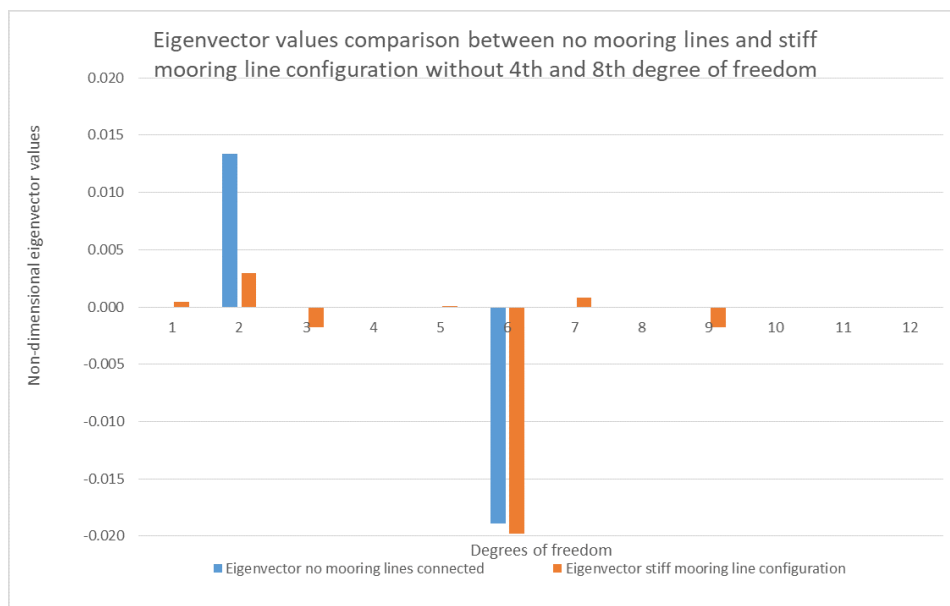
Figure 5.13: Eigenvector value comparison between the multi-body system without mooring lines and the multi-body system with a stiff mooring line configuration, configuration 3 in figures 5.10 and 5.11. The natural frequency that is compared is the natural frequency at \blacksquare rad/s . In this figure the eigenvector values of the vessel roll and cargo sway motion are neglected
