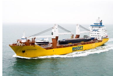
(b) BigLift's Happy-D type vessel. A vessel with 2 cranes of 400 mton and 1 crane of 120 mton.
