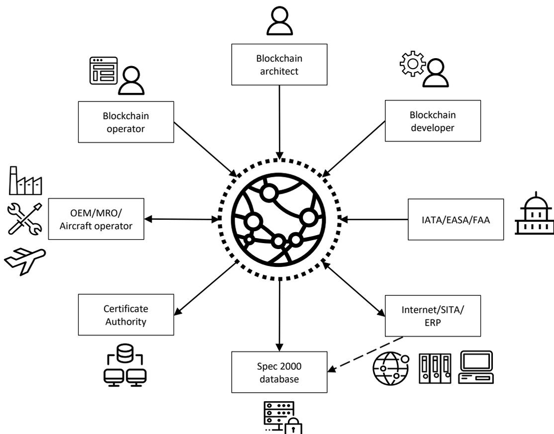
Figure 17 – A Blockchain-based aircraft spare part ecosystem
