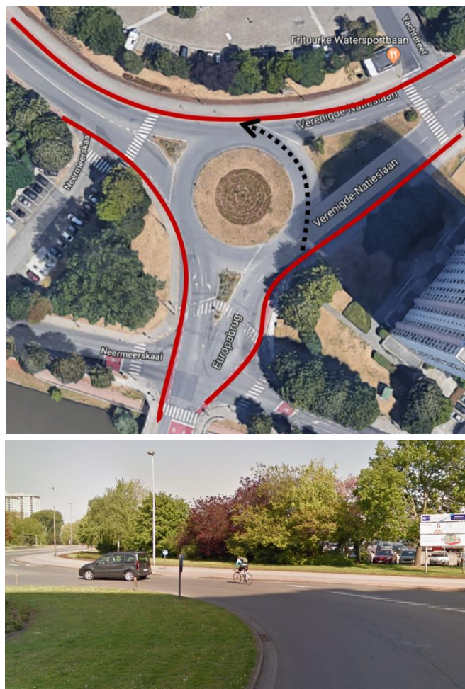
Figure 38. Illustration of the path (black dotted arrow between red cycleways) that cyclists make to turn left on a roundabout (top) and an image of a cyclist making that crossing maneuver on that same roundabout. Source: Google Maps.
