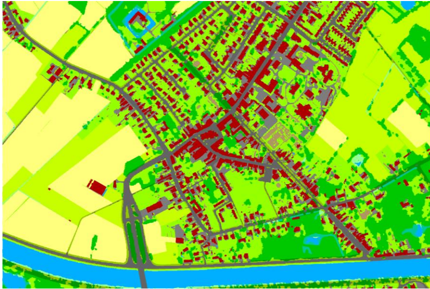
Figure 8. Impression of the land use raster data obtained from the GRB with different types of vegetation (each different shade of green representing), buildings (red), water (blue), roofless built areas (brown) and streets (grey).
