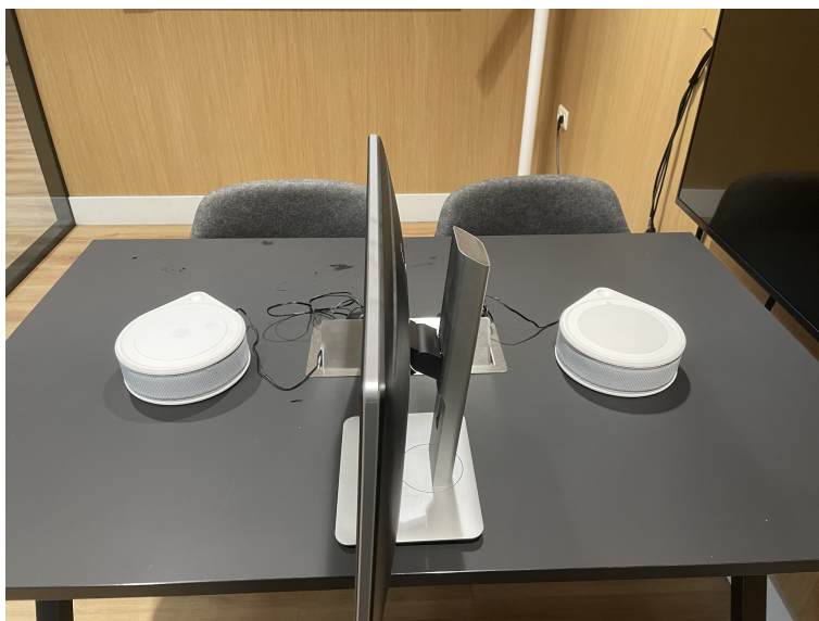
Figure 5.5: The experimental setup in a meeting room in TU Delft. Two speakers are used to play the testing samples.
