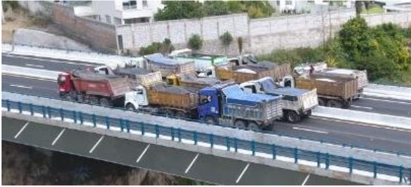
Figure 11. Load application with dump trucks.
