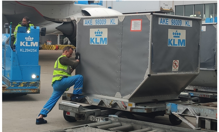
figure 1.1 Personnel putting a lot of effort into getting a container onto a dolly
