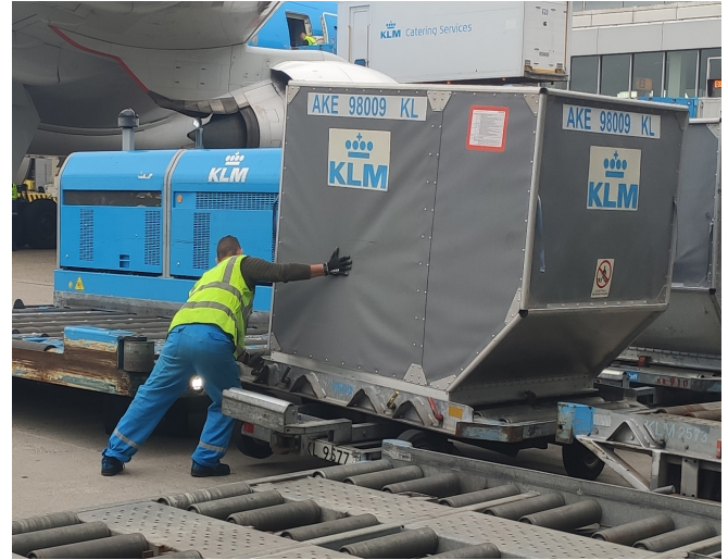
Figure 10.2 - The current situation also requires the opening of the lock manually
