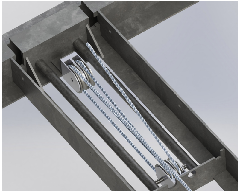
Fig12.16. Pulley with the 6mm cable
