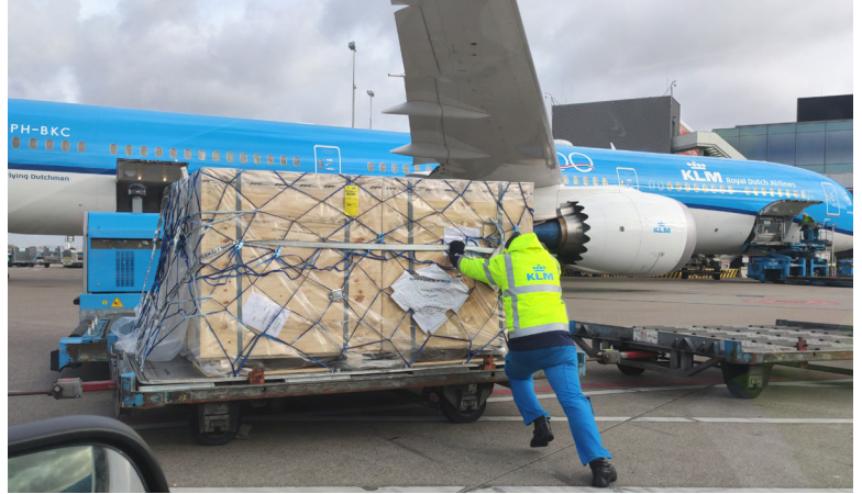
Figure 8.9- Pallets also have to be pushed manually onto the transporter
