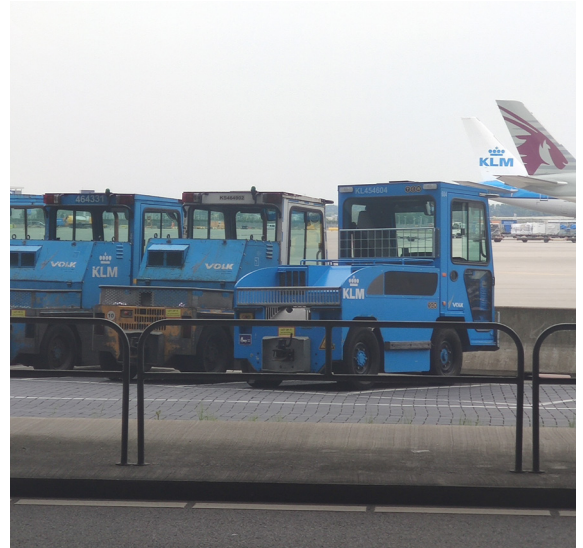
Figure 3.15. On the right the new Volk electric tractor and on the left the old Volk diesel tractors
