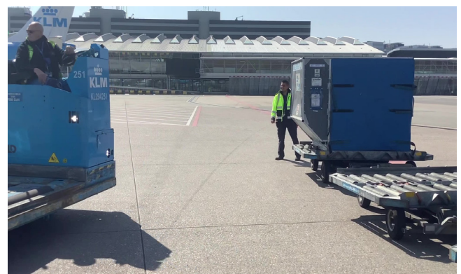
Fig 6.4. The pusher has to wait for the transporter to reach the second container
