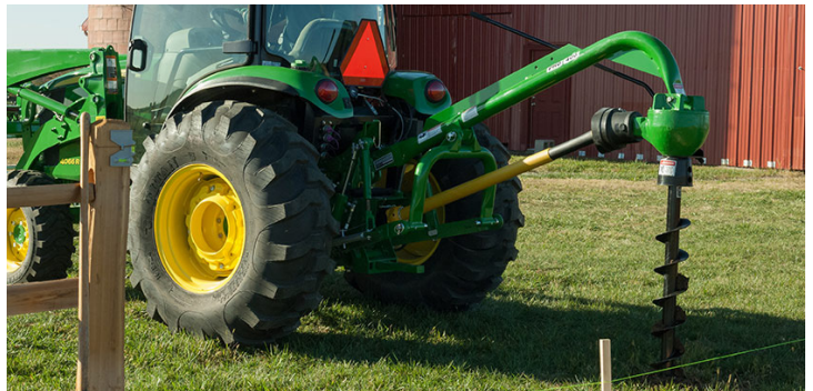
Secondary axle of a tractor powering a drill
