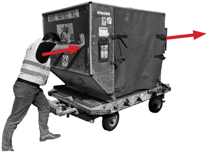
Figure 10.1 - In the current situation a push from the personnel is needed to move a container
