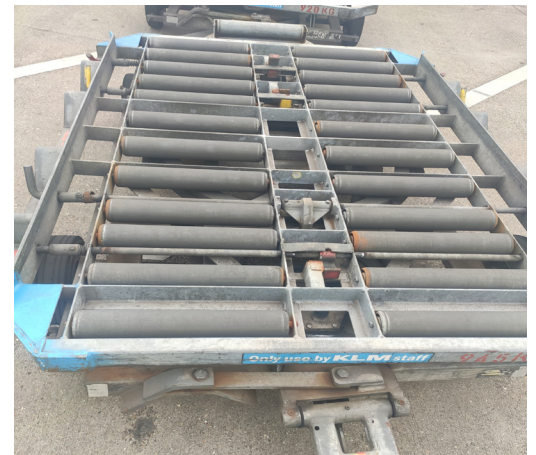
Fig 3.9. The current version of the 5ft dolly has 25 rollers in total. For the new dolly the single roller on the back will be removed and the rollers will be placed further apart that only 20 rollers are needed
