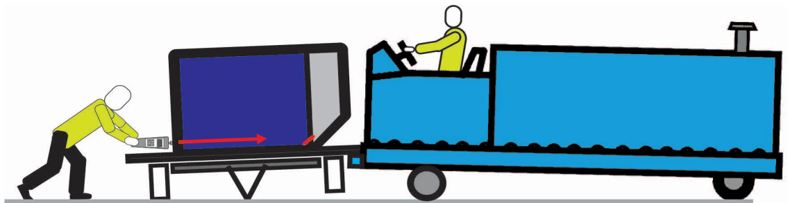
The transporter lifts the dolly and the container is pushed with the gauge
