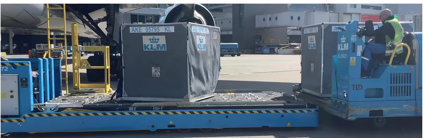
Fig 6.6. Rotating a container on the loader .
