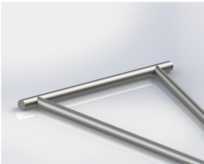
Fig12.4 The head of the sled, with the axles for the hooks
