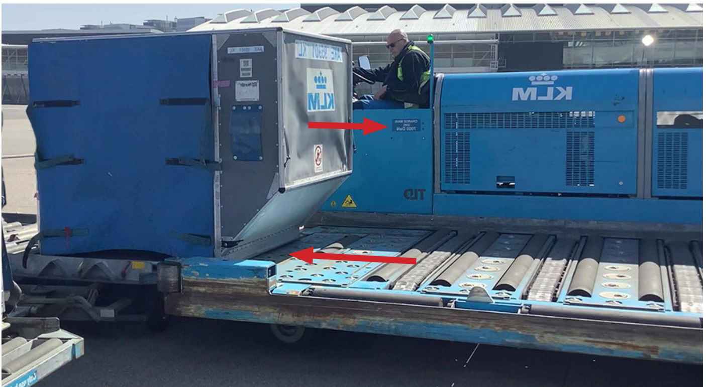
Figure 10.3- In the new situation the transporter pushes to move a container without the need to open the lock
