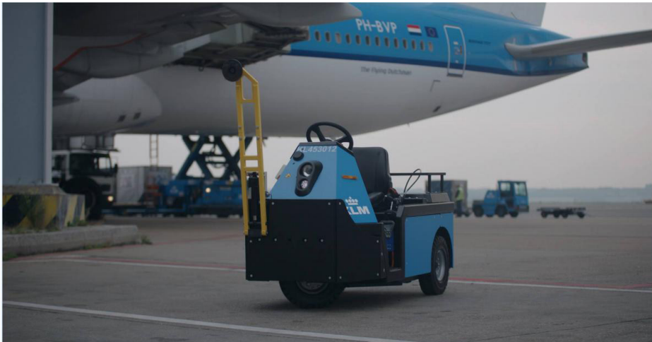
Figure 3.28. Push assist created by KLM and produced by Spijkstaal (Spijkstaal, 2018)
