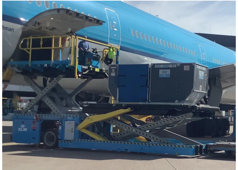
Figure 3.20. TLD TXL-838-reGen loading containers into an aircraft
