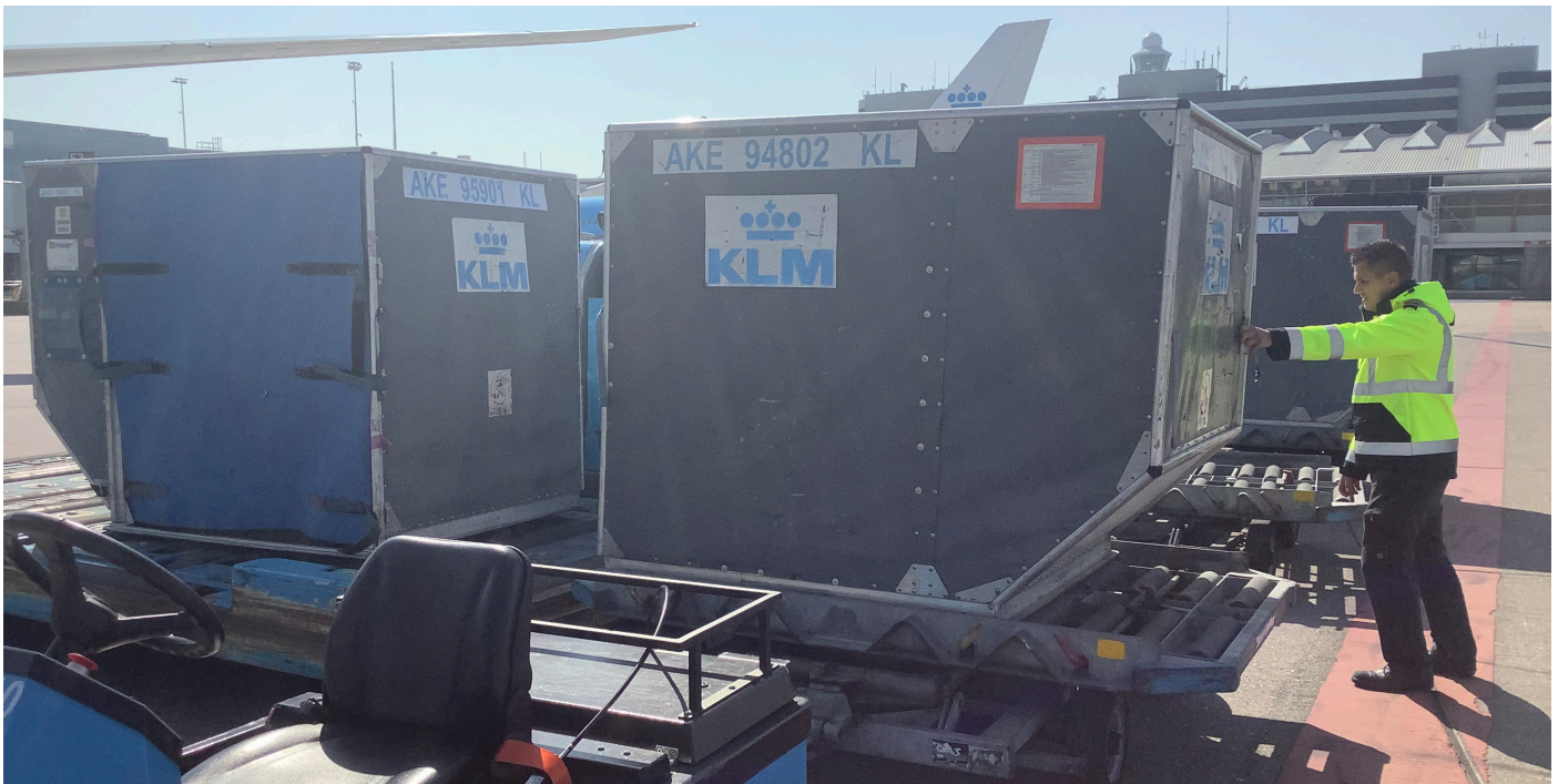
Fig 5.4. Personnel has to stand on the red clearance line to be able to push a container
