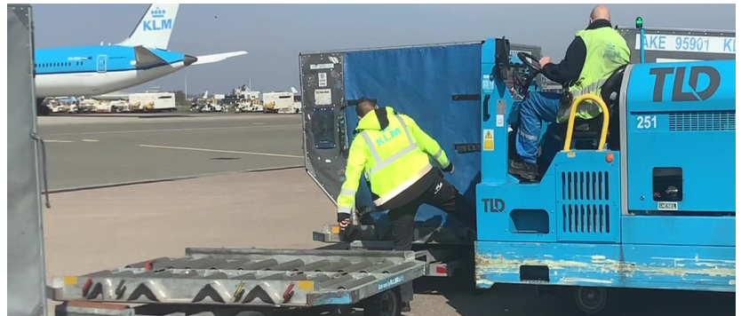
Fig 8.2. The employee has to stand close to a moving transporter to open the locks.
