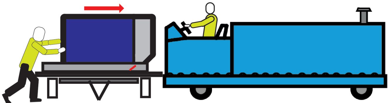
Fig 4.12. Pushing the container onto the transporter.
