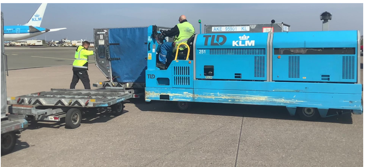
Fig 4.15. Pushing the second container onto the transporter
