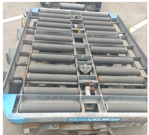
The rollers have a specific friction that give a reaction force on the container when pushing it
