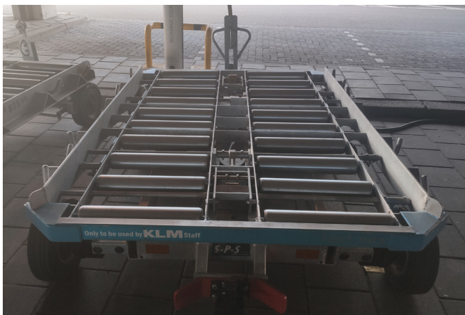
Fig 3.8. The new version of the 5ft dolly has 20 rollers in total and less structural members
