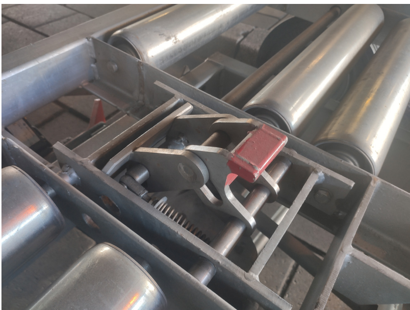
The automatic lock is still in development. In the future all dollies will have this kind of lock.
