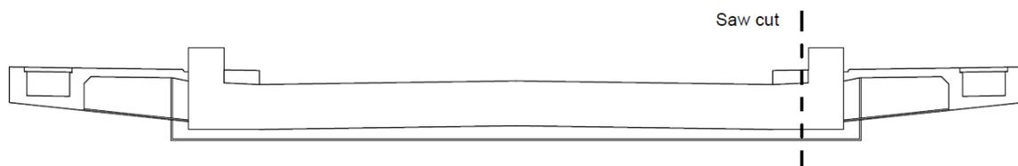
*Figure 3.8: Cross-section of the bridge with the position of the saw cut*
