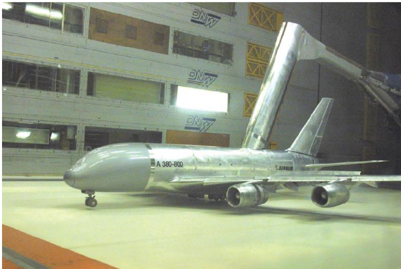
Fig. 2-7. An aircraft model with TPS tested in a wind tunnel [32].
