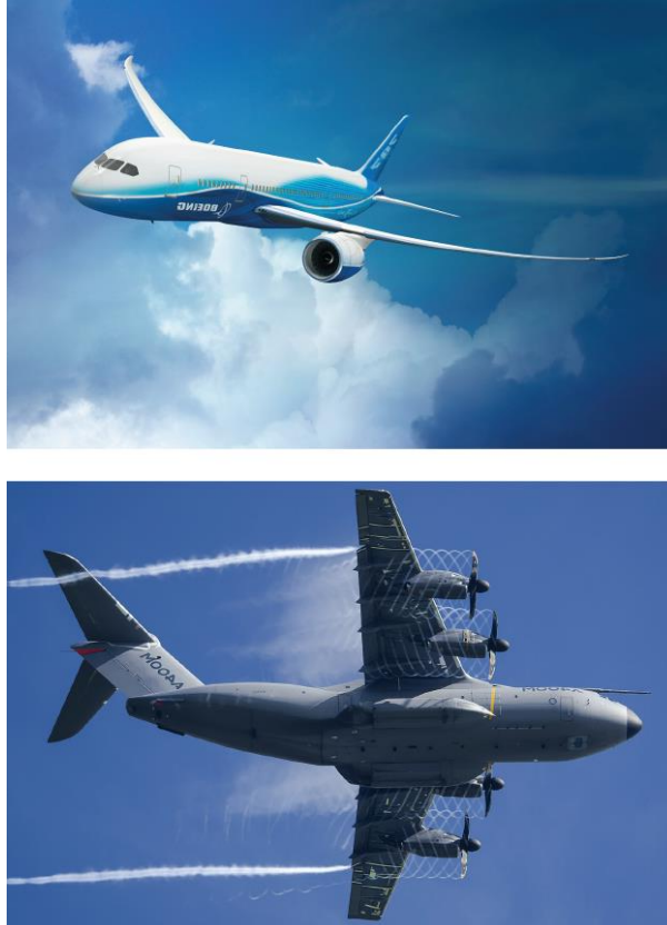
Fig. 2-3. Modern turbofan (top) and turboprop (bottom) engine aircraft commonly place the propulsion system underneath the wing (Courtesy: Boeing and Airbus).
