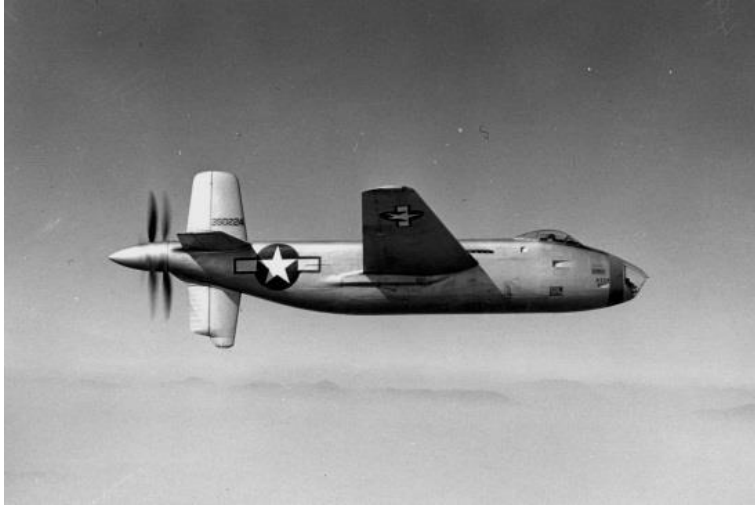
Fig. 2-14 XB-42 in 1944 showing the integration of fuselage and counter-rotating pusher propellers [76].
