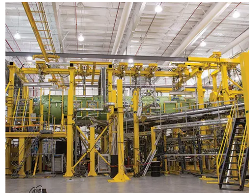
Figure 9.16: Fuselage stress test at Gulfstream, done by clamping the midsection[40].
