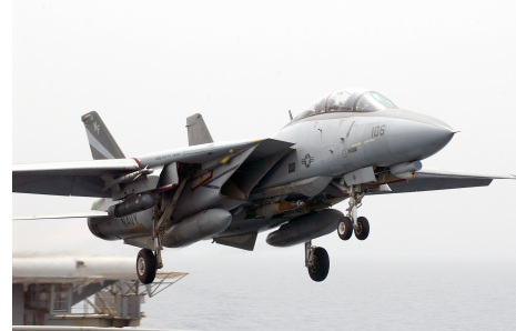
Figure 8.11: Ramp inlets on an F-14 Tomcat for supersonic flight regimes 7
