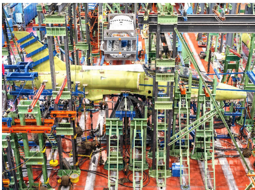
Figure 9.15: Fuselage stress test of an L-39 Albatross with a pivot point[39].
