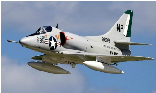
Figure 8.10: Fuselage embedded inlets on a subsonic A-4B Skyhawk[25]
