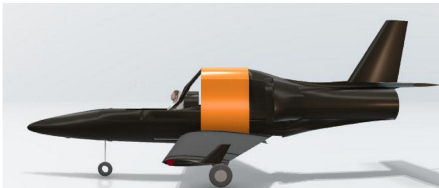
Figure 9.20: Fuselage cross-section used for analysis, highlighted in orange (indicated with the green lines in Figure 9.18 and Figure 9.19).
