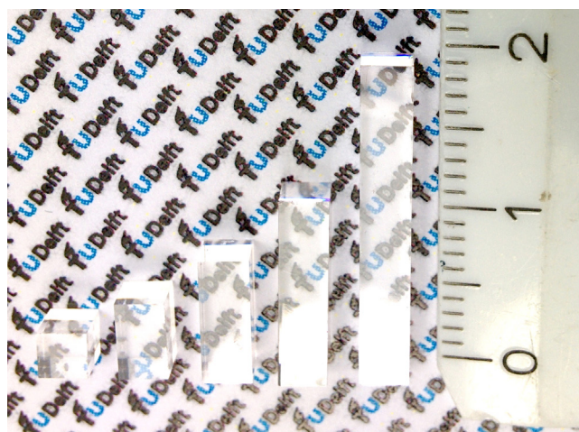
Figure 4. Photograph of the BGO samples tested in this work. All crystals have a cross-section of 3 mm \times 3 mm. From left to right, the crystal lengths are 3 mm, 5 mm, 8 mm, 12 mm, and 20 mm.
