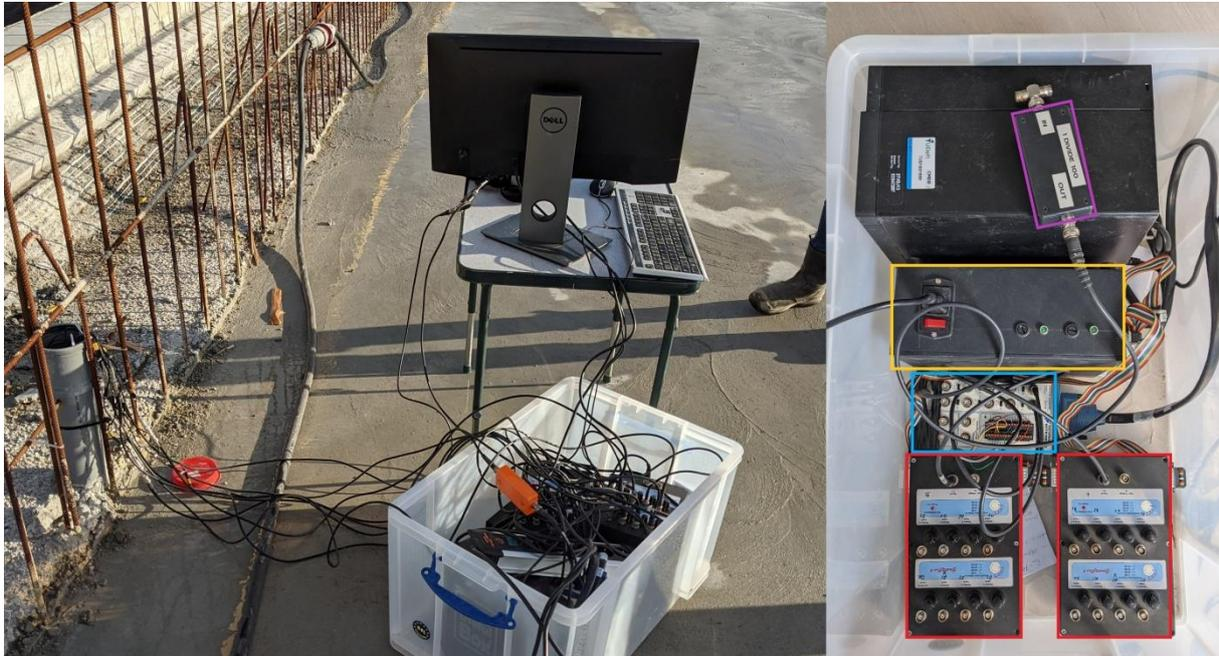
**Figure 10: Measuring setup on site (left) with the MUX system contained in a plastic box (right) with the voltage divider (purple), power supply unit (yellow), connector (blue) and MUX channels (red)**
