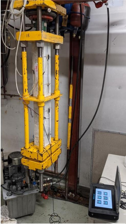
Figure 16: Creep test setup of two geopolymer samples with embedded SA loaded in tandem
