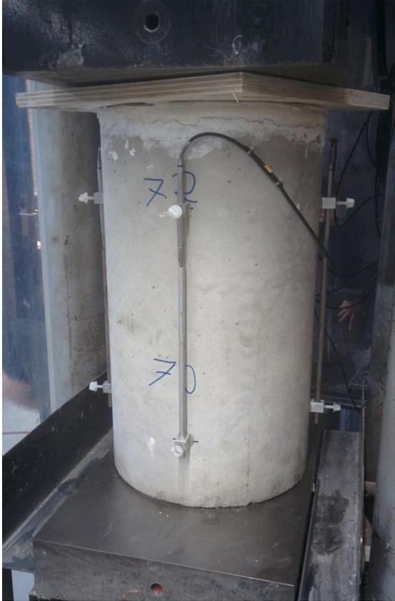
Figure 15: Compression stress test setup of a concrete cylinder with embedded SA
