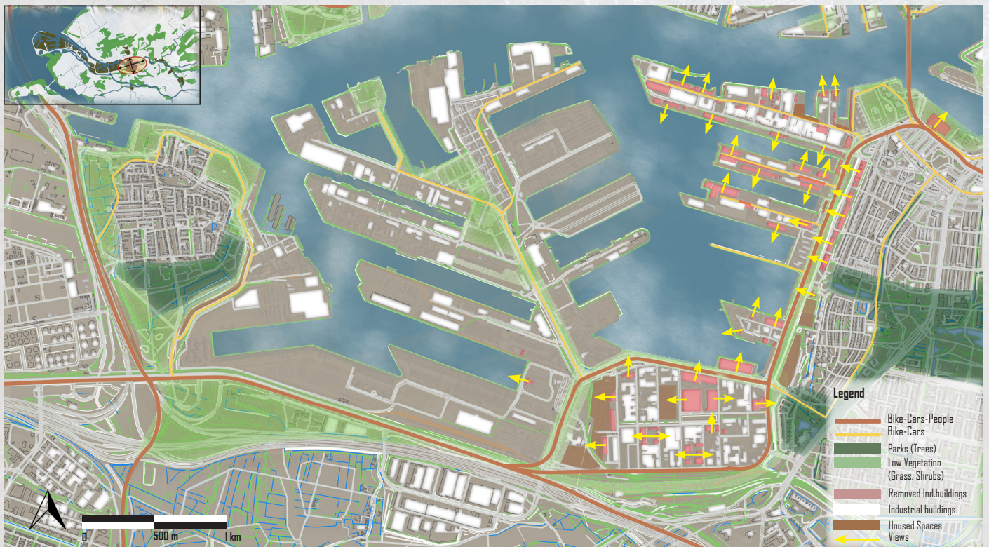
Figure 74. Masterplan of the actual area of intervention: Waalhaven and surroundings. Removal of obstructing industrial buildings.
