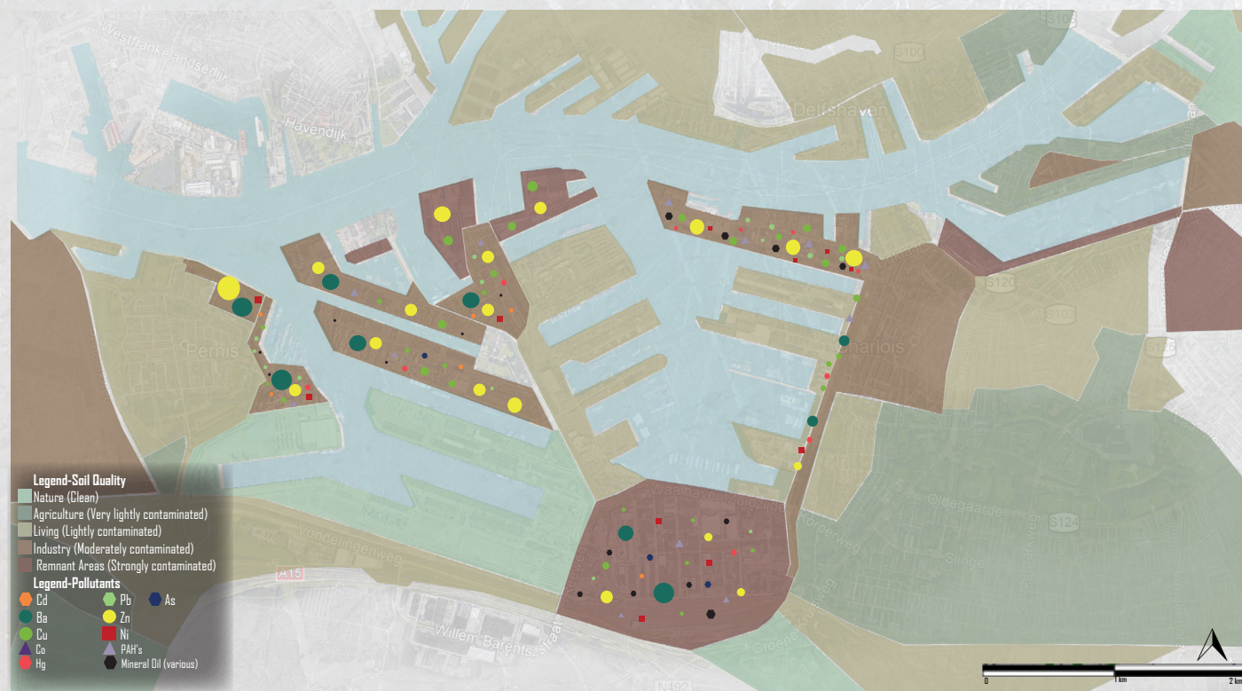
Figure 59. Map showing Soil Pollutants in Waalhaven area. The most frequent ones are Zn, Ba. In second place, Cu and Mineral Oils.
