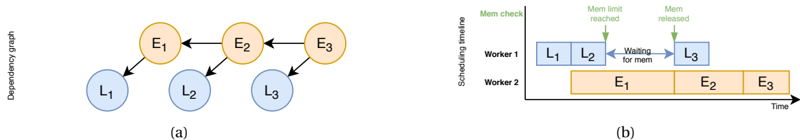
Figure 6.6: MASA scheduling a 3-layer DNN on 2 workers. Subfigure (a) shows the dependency graph. The scheduler introduces an idle period for worker 1 to prevent memory paging as is shown in subfigure (b).
