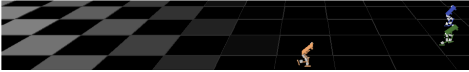
Figure 5.8: This figure illustrates the performance of \pi^{\text{idl}} (yellow), \pi^{\mathcal{D}} (green), and \pi^{\text{true}} (blue) on the true model. The policy learned with the difference model achieves almost the same walking distance while only requiring 6.5% of interaction time compared to the cold-started method. Also see supplementary video.
