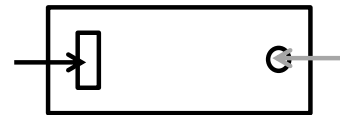
Figure 42: Moment arm produces radial force on the external part of the coupling. Resultant force exerted by the axle is shown in gray.
