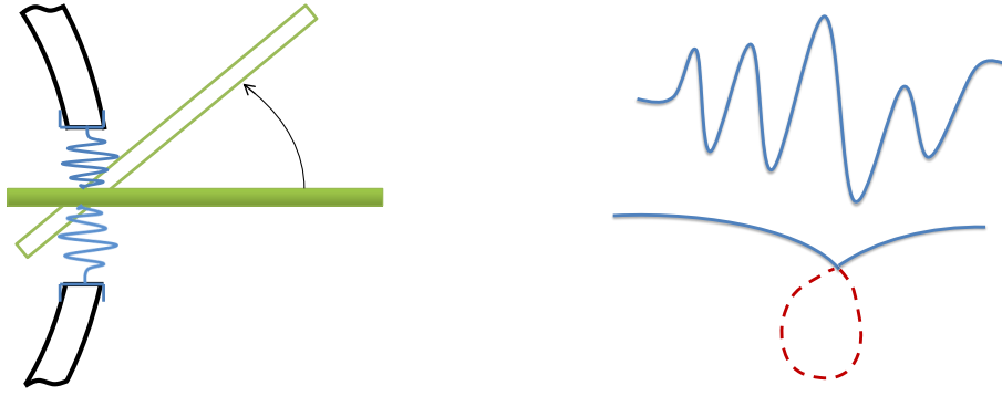
(a) Simple representation of how a flexure could be used as a hull. Black is the solid hull of the vehicle, green the fin and blue the flexure.
