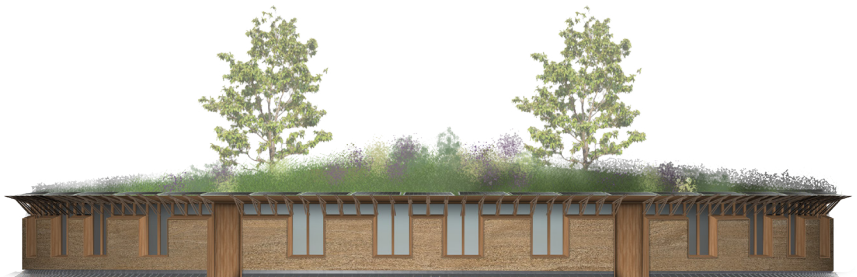
The complete facade with an overhang to hold back the water. (Own work)
